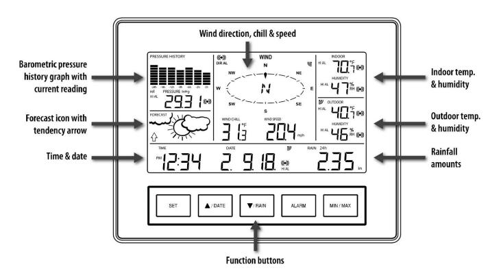
When the signal from an outdoor transmitter is successfully received by the Weather Station, the corresponding \(\mathbb{E}\) icon will be switched on. (If not successful, the \(\mathbb{E}\) icon will not be shown on the LCD). The user can see whether the last reception was successful (\(\mathbb{E}\) icon is on) or not (\(\mathbb{E}\) icon is off). Blinking of the \(\mathbb{E}\) icon shows that a reception is in process.
